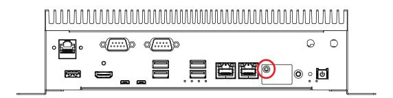
Step 2 Inserting SIM card, make sure the system power is not plugged.
