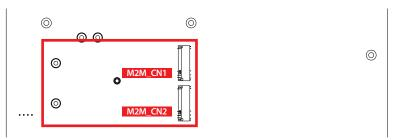
M.2 key M connector is suitable for applications that use Host I/Fs supported PCIe x4, like w NVME Module card types include 2280.
