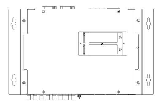
Step 3 Install M.2 Key M 2280 into slot and fasten one pan head M3x4L screw.
