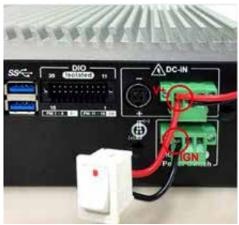
For testing purpose, you can refer to the picture blow to simulate ignition signal input controlled by a latching switch.
