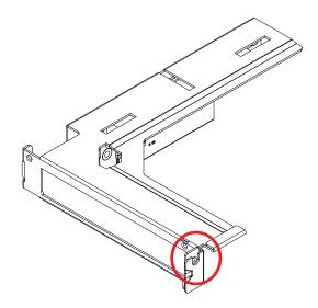
Step 4 Install PCIe card and fasten the screw indicated.
