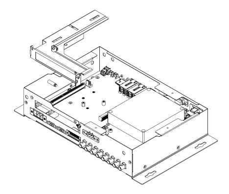
**Step 3** Remove the screw indicated and separate I/O bracket from assembly Riser Card.
